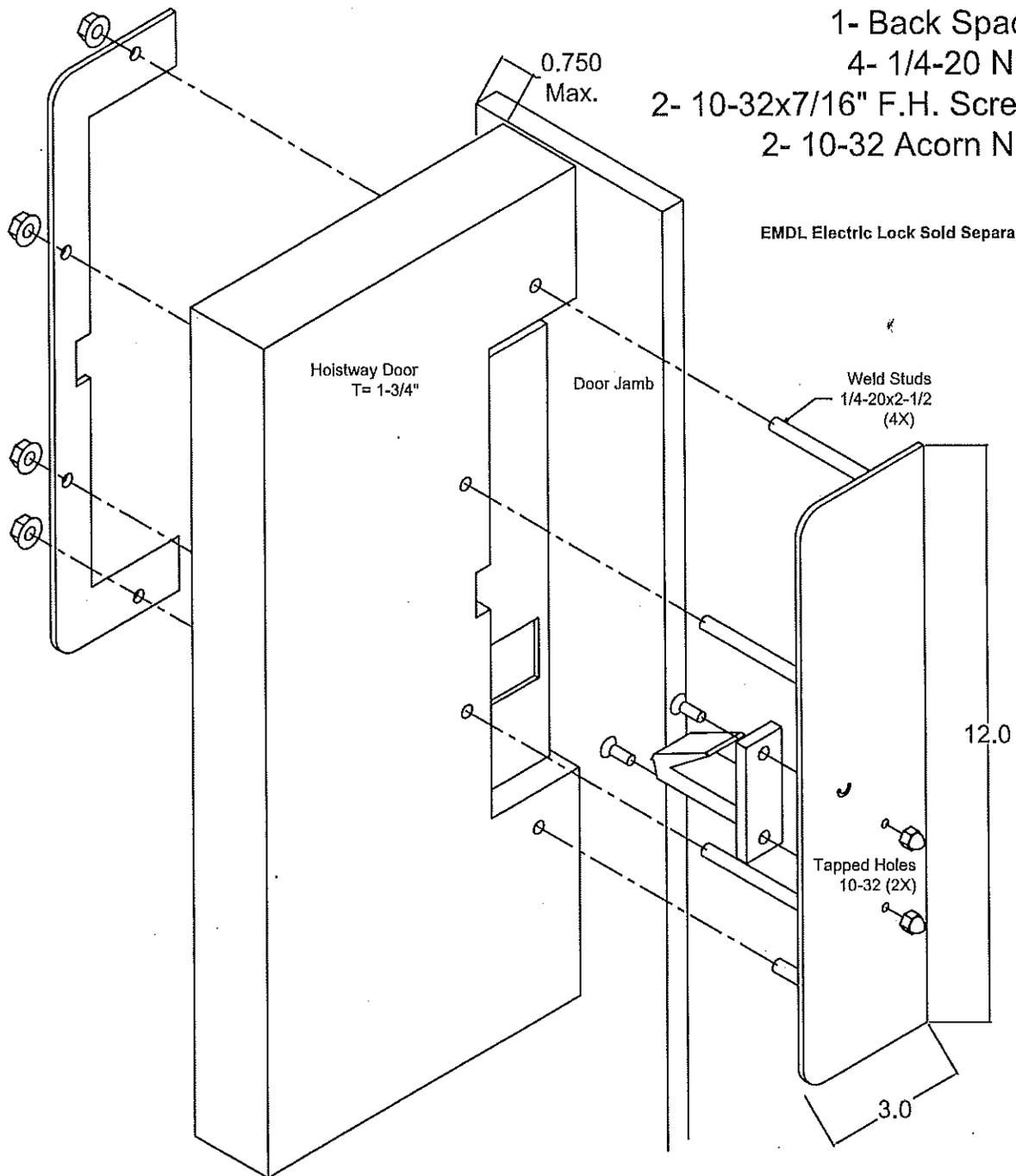
Note: If Hoistway Door is less than 1-3/4" thick additional 1/8" spacers are required on Hall side of plate. Additional spacers are sold separately. Part Number: EMDL750SP
