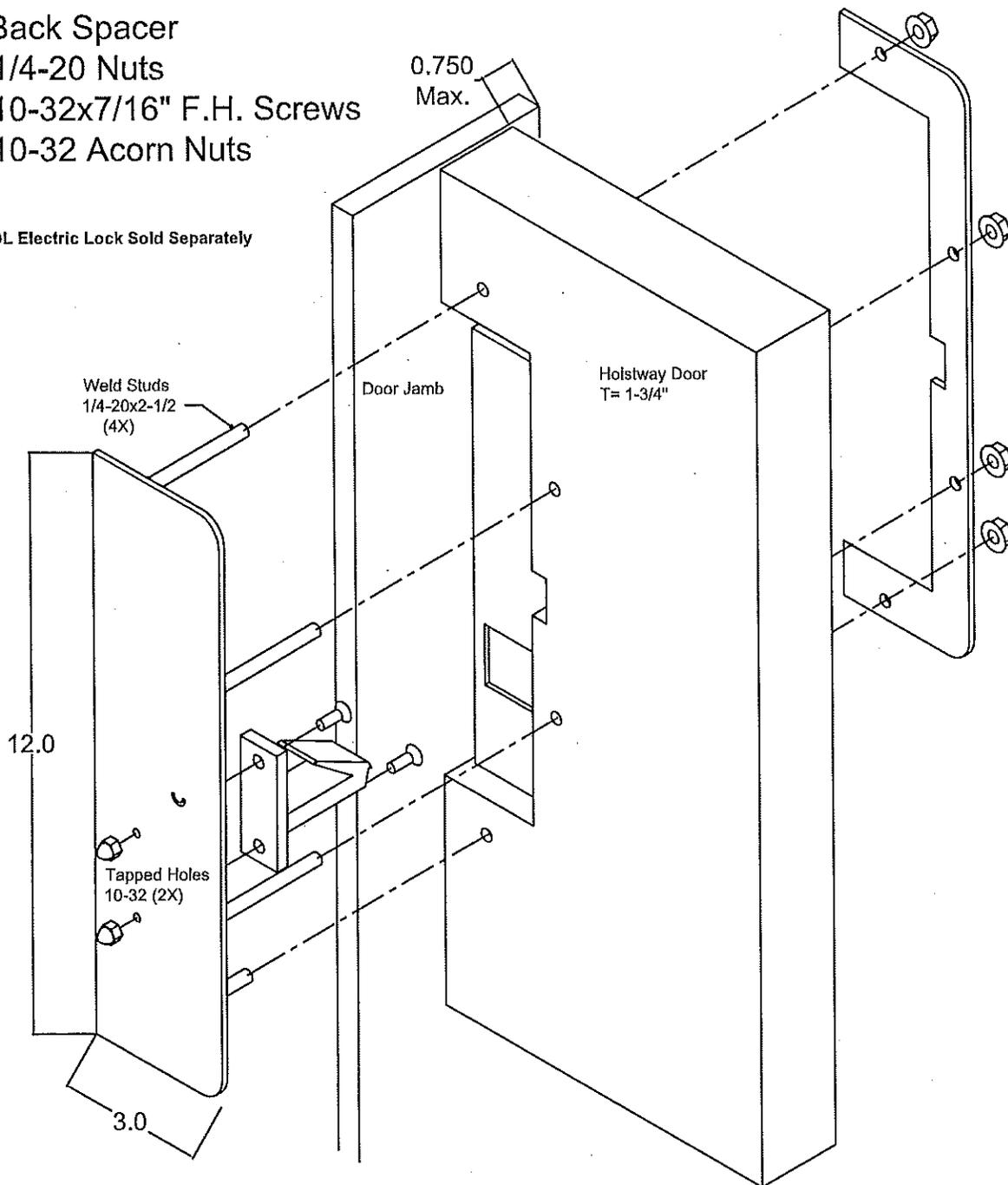
Note: If Holstway Door is less than 1-3/4" thick additional 1/8" spacers are required on Hall side of plate. Additional spacers are sold separately. Part Number: EMDL750SP
