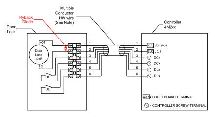
Note: DO NOT USE "THERMOSTAT" WIRE Hoistway wire must be stranded.
