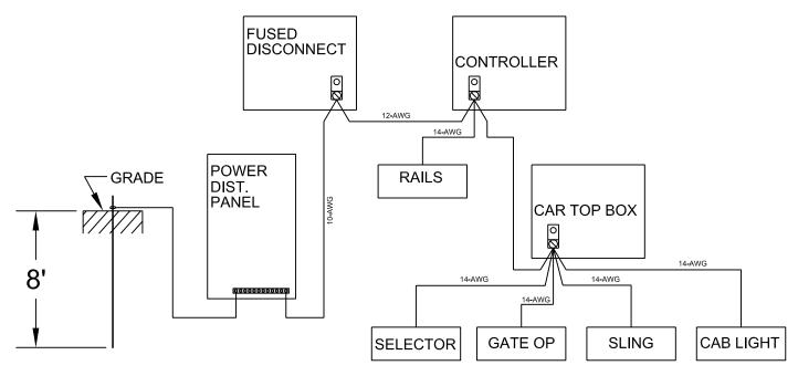
Note: All Ground wires must be stranded wire
